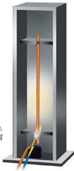
Test of vertical flame propagation, self-extinguishing
