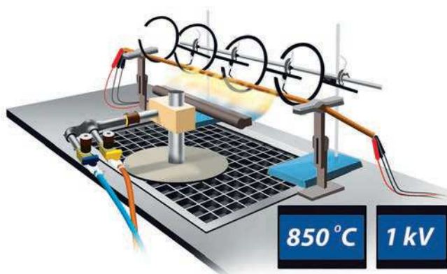
Testing according to EN 60331 (850°C 1 kV)
