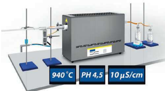
Measurement of the corrosiveness of the combustion gases
